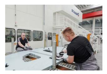
Image 2 (fri201841910.jpg): Stahlo Stahlservice produces customised shaped blanks with special surface quality at its Gera site on one of Europe's largest blank cutting lines, and it can process ultra-high-strength steels with a tensile strength of up to 1,900 MPa.
